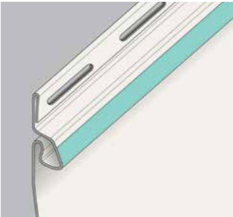
The unique TriBeam system gives Charter Oak superior rigidity, helping to ensure straight course lines and even walls, on both new and existing homes. The result is a particularly beautiful installation with the built-in strength to maintain an enduring appearance.
