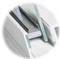
**The Optional Foam Spacer** combines a structural foam spacer with a seal of hot melt butyl to create a "warm" non-conductive edge. This non-metal design eliminates any metal-to-glass contact, thereby increasing the edge of the glass temperature by more than 16° – resulting in 60% more energy efficiency than a traditional box metal spacer.
